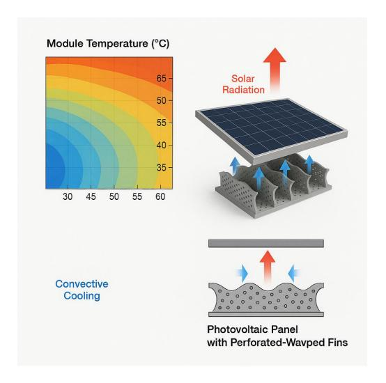
• Average PV Temperature: The average PV module operating temperature for the novel heatsink might be 45,°C, while for a conventional flat-finned heatsink, it could be 55,°C, and for an uncooled module, it could reach 65,°C (Figure 1b). This demonstrates a substantial reduction in operating temperature due to the optimized fin geometry.
