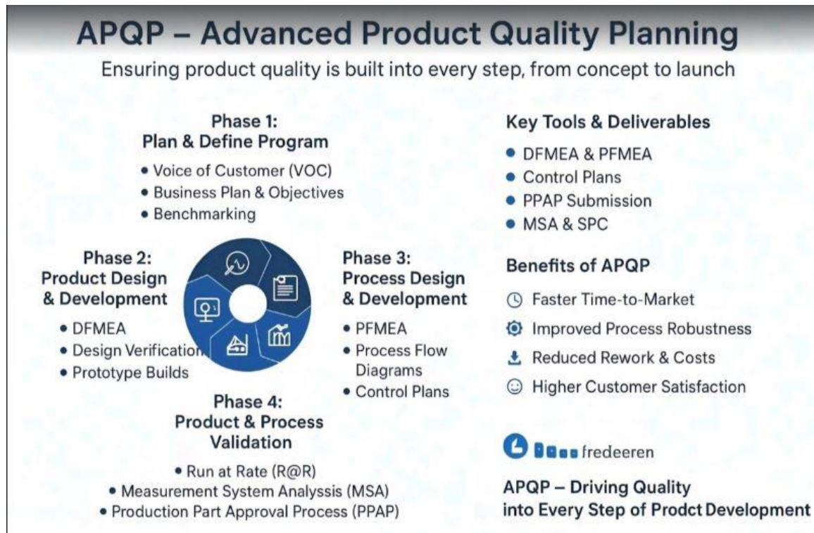
Figure 1 APQP phases linking PPAP elements to product and process development in automotive quality management.
